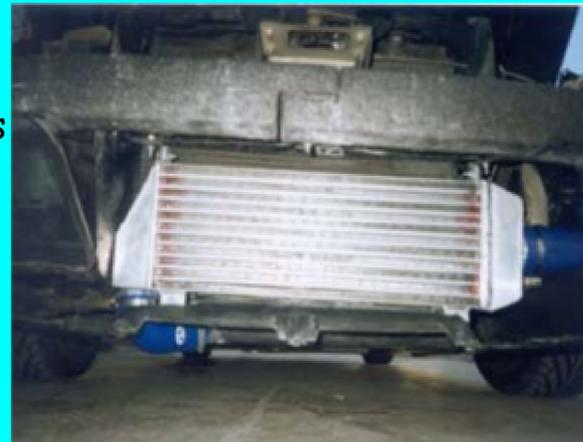
The outlet of the turbo compressor is fed to the left hand side of the intercooler via silicon hoses and aluminium piping. To do this a small section of the plastic undertray needs to be cut out to let the turbo pipe exit through and to the side of the intercooler. The blue pipe in the centre of the image is the silicon hose connected to the turbo compressor outlet.
